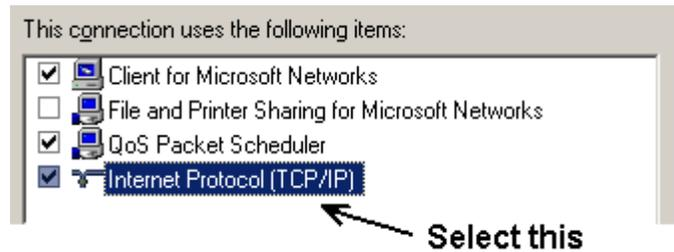
Note: If you have multiple Ethernet cards, you may have multiple lines labeled "TCP/IP --> Ethernet card". Locate the Ethernet card that corresponds to the physical connection to the AcquiLite and then select the TCP/IP option that is linked with that Ethernet card.
