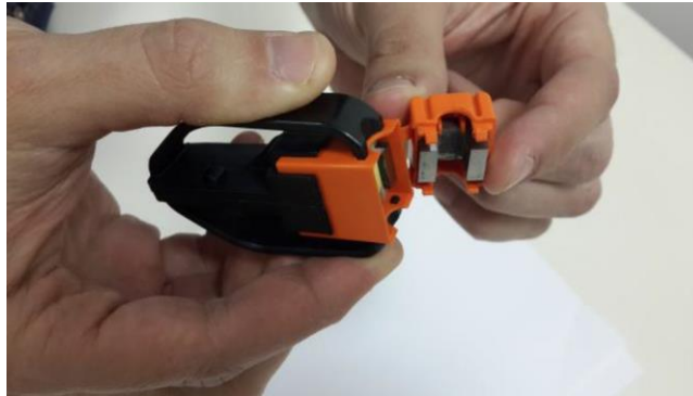
Figure 5. Press the opener to release the cover.
