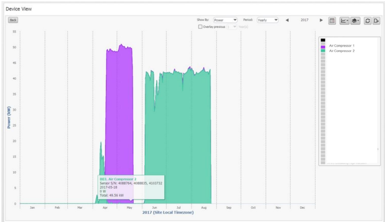
Figure 5. Site Air Compressor 1 and 2 Monthly Energy Usage Comparison, Device Level View
